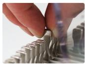
QSA (Quick Size Adjustment) technology means that punching pins can be cancelled and paper formats can be changed quickly and easily.<sup>(1)</sup>
