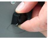
Depth gauge feature allows the operator to adjust the punched hole margin from 2 mm to 4,5 mm<sup>(1)</sup>. This adds strength to the bound edge.
