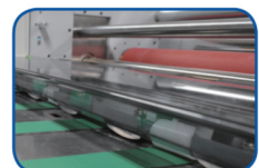
AUTOMATIC FEEDING GAP CONTROL DEVICE
