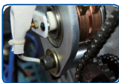
THERMO-Couple Inserted FOR TEMP. SENSING
