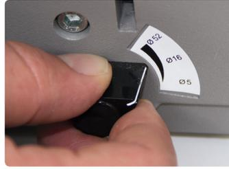
The depth gauge feature allows the operator to adjust the punched hole margin from 2 mm to 4,5 mm<sup>(1)</sup>. This adds strength to the bound edge.
