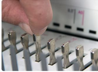
QSA (Quick Size Adjustment) technology allows the punching pins to be cancelled and the paper formats to be changed quickly and easily.<sup>(1)</sup>
