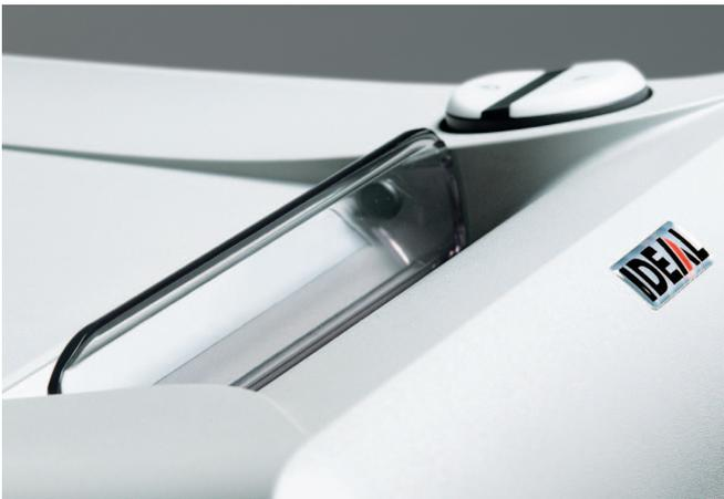
**SAFETY PROTECTION SYSTEM** Extremely safe: electronically controlled safety flap in the feed opening to keep fingers, ties or other objects away from the cutting shafts.
