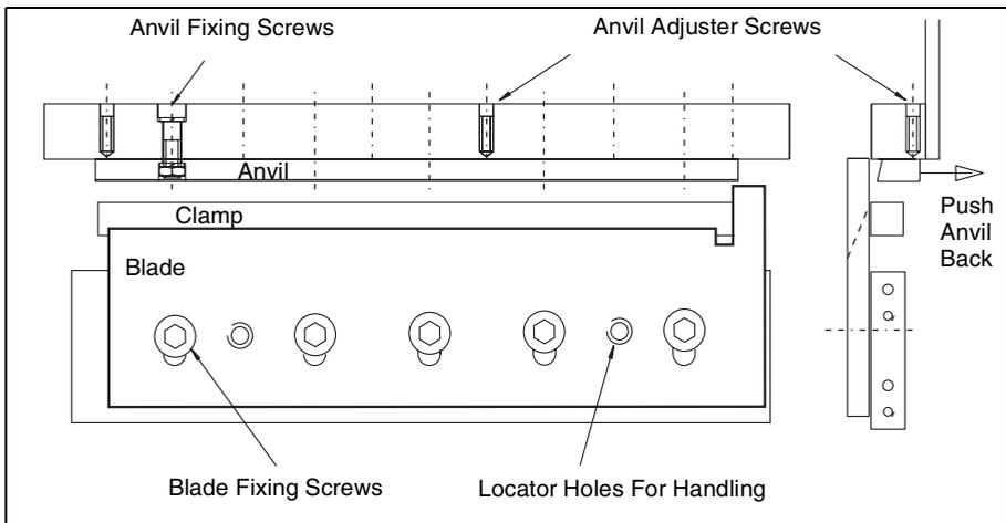
FIGURE 37 ATR Blade Removal
