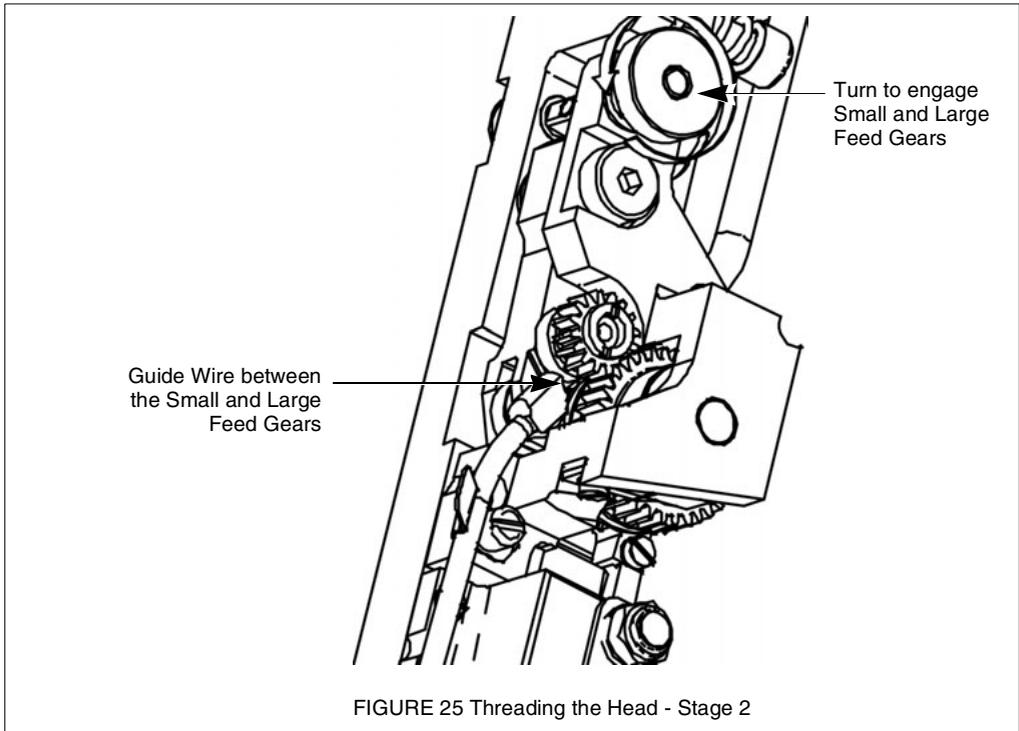
Cycle the heads to cut the wire to the correct length.
