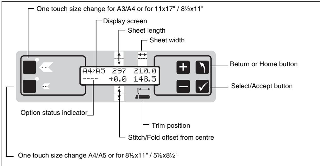
FIGURE 39 Offline Control Panel (metric measurements shown)
