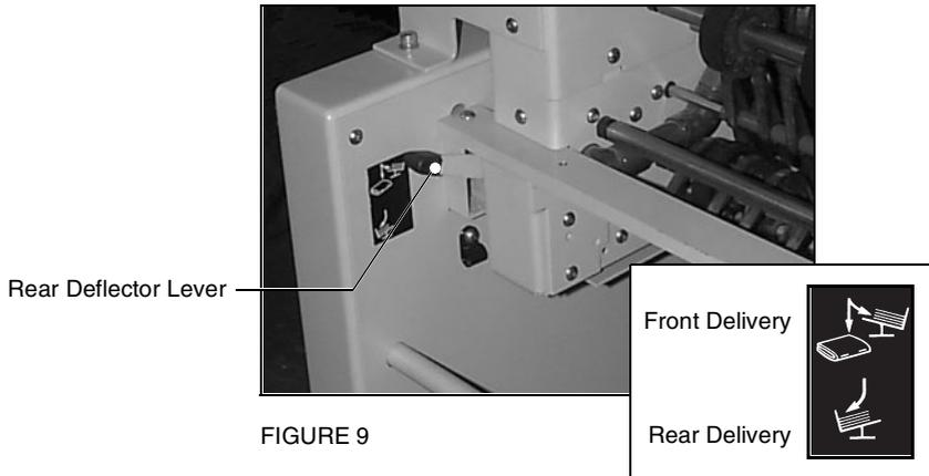
**DigiVAC+:** Set the delivery lever to its upper position, to deliver sets to the rear.
