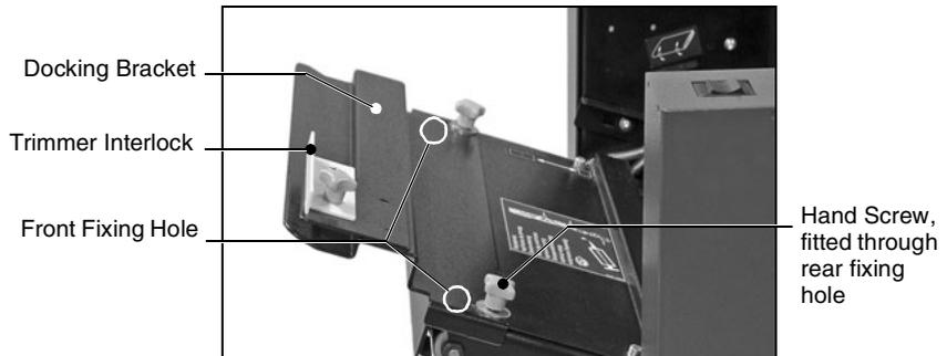
FIGURE 36 Docking Bracket (shown mounted in the standard position)
