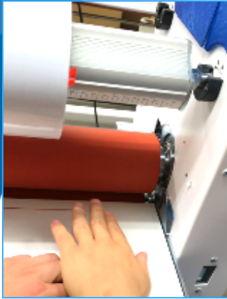
Safety sensor High sensitivity sensor prevents finger pinch
