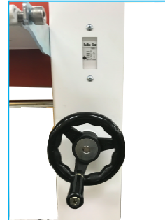
Easy operation handle - Roller clearance
