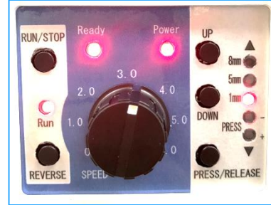
Easy operation panel - Speed/pressure adjustment - Run/stop, reverse mode
