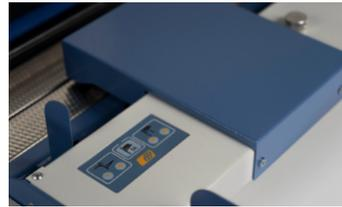
High pile suction feeder for paper stack up to 10cm.
