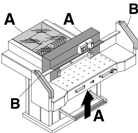
All components which may endanger the operator are covered by a guard (A).
