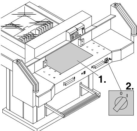
Remove all tools and distribute paper along the entire cutting length (1.). Turn main switch to position "I" (2.).
