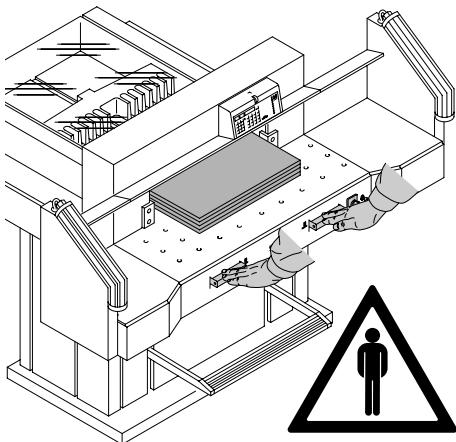
The machine is designed for cutting stacks of paper to a specified size.
