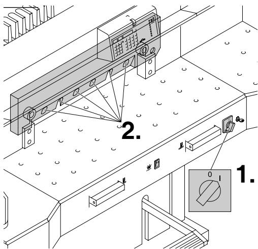
Turn main switch to position "I" (1.). Blade will return to upper position. Tighten 6 blade screws (2.) firmly.
