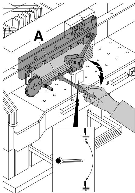
Paper cutting test. If the last sheet or several sheets are not completely cut, gradually turn the blade depth adjustment (A) 1/12 downwards until all the paper is completely cut. Do not set too low as blade will become blunt sooner.
