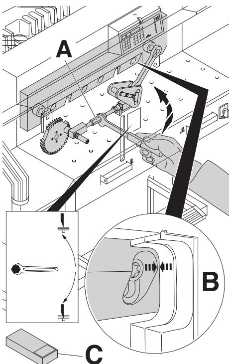
Turn the blade depth adjustment (A) towards the top until the blade screw recess corresponds with the frame recess (B). (Spanner found in tool set (C)).
