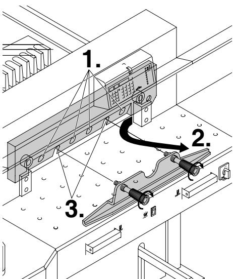
Lightly tighten 4 of the 6 blade screws with washers (1.). Remove the blade changing tool (A) (2.). Lightly tighten the remaining blade screws with washers (3.).
