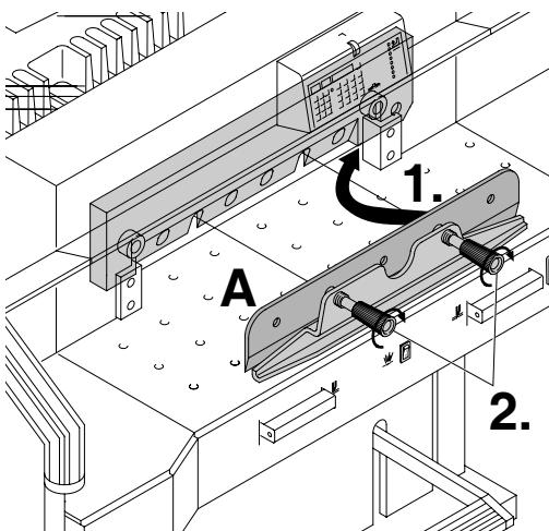
Place the blade to be exchanged with the blade changing tool (A) mounted (1.), into the blade carrier and push it up to the top and screw it into place with the grips (2.).
