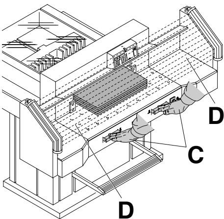
The cutting action, which is dangerous to the operator, is protected by a two-handed control system (C) and safety beam guard (D).
