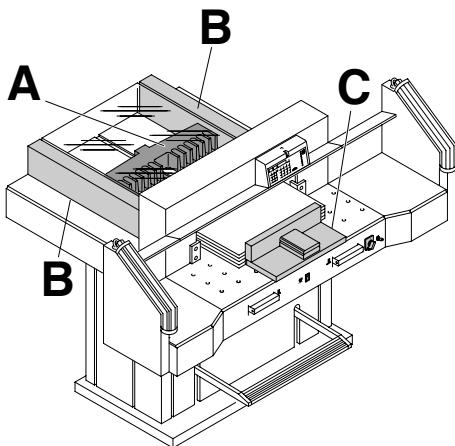
Position the paper on the backgauge (A) and side lays left or right (B).
