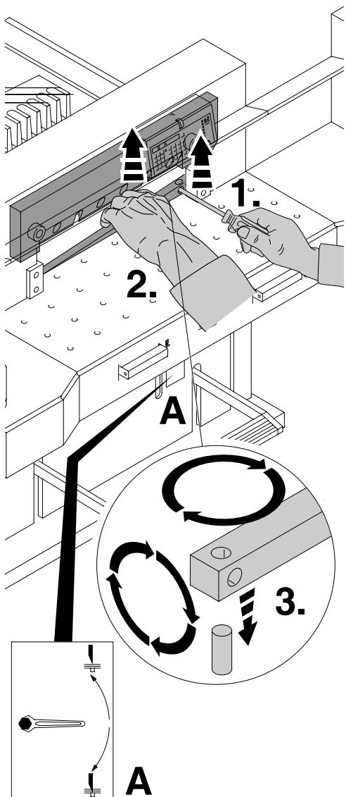
Take out the cutting stick with a small screwdriver. If needed the cutting stick can be turned or exchanged. (The cutting stick can be used eight times).
