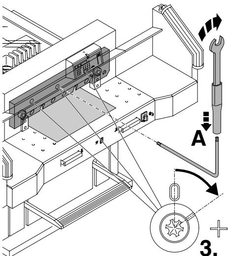
With the special wrench (A) the 3 eccentrics should be screwed down until the paper is cut along the entire length of the blade (3.) (The blade must remain parallel, not too deep into cutting stick).
