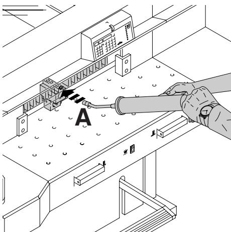
Grease the backgauge (A) control weekly with a grease gun. Advance the backgauge as far as possible to the front. (Use non-resinous oil or grease).
