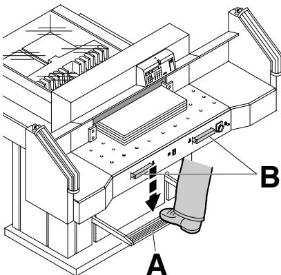
The clamp moves automatically when cutting is activated.
