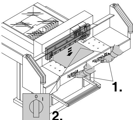
Lower the blade by pressing both cutting buttons (1.). Keep one button pressed and turn off the main switch (2.).
