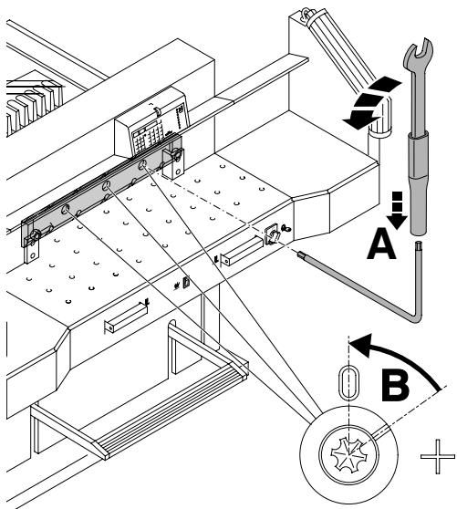
The 3 eccentrics are now exposed and should be turned counter clockwise to position "0" with the special wrench and attachable extension pipe (A) (in the tool set). The slot must correspond to position "0" (B).
