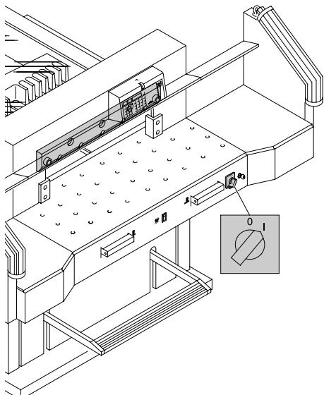
Remove the special wrench and turn on the main switch until the blade returns to the home position.
