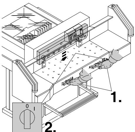
Lower the blade by pressing both cutting buttons (1.). Keep one button pressed and turn off the main switch (2.).
