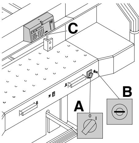
Position the main switch to "I" (A). Insert the key for the control system and turn it to the right (B).
