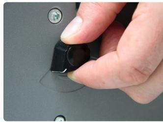
Depth gauge feature allows the operator to adjust the punched hole margin from 2 mm to 4,5 mm<sup>(1)</sup>. This adds strength to the bound edge.
