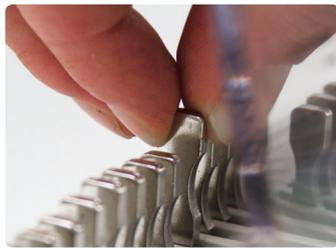
QSA (Quick Size Adjustment) technology means that punching pins can be cancelled and paper formats can be changed quickly and easily.<sup>(1)</sup>
