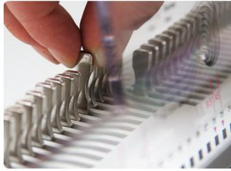
QSA (Quick Size Adjustment) technology means that punching pins can be cancelled and paper formats can be changed quickly and easily.
