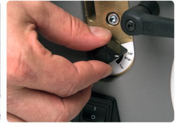
The depth gauge feature allows the operator to adjust the punched hole margin from 2 mm to 4,5 mm<sup>(1)</sup>. This adds strength to the bound edge.
