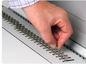
QSA (Quick Size Adjustment) technology allows the quick cancellation of punching pins without the need to remove the die.
