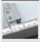
The accurate backgauge and side lays are made from cast aluminium and allow a precise alignment of the paper stack
