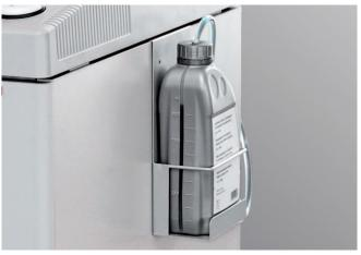
**ELECTRONIC OIL INJECTION** IDEAL 3105 and IDEAL 4005: the automatic oil injection system lubricates the cutting shafts when shredding and guarantees a consistently high shred performance.
