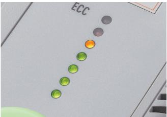
**ECC - ELECTRONIC CAPACITY CONTROL** ECC - Electronic Capacity Control indicates the used sheet capacity during shredding process to avoid paper jams.
