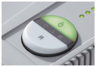
**EASY\_SWITCH** Innovative multifunction control element with integrated optical signals for the operational status.
