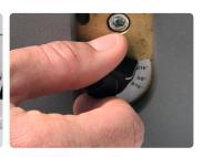
The depth gauge feature allows the operator to adjust the punched hole margin from 2 mm to 4,5 mm<sup>(1)</sup>. This adds strength to the bound edge.
